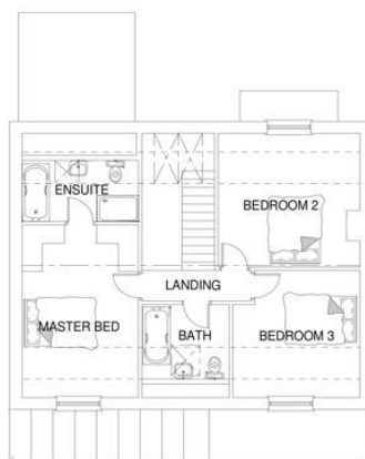
PROPOSED FIRST FLOOR PLAN (scale 1:100@A3)
